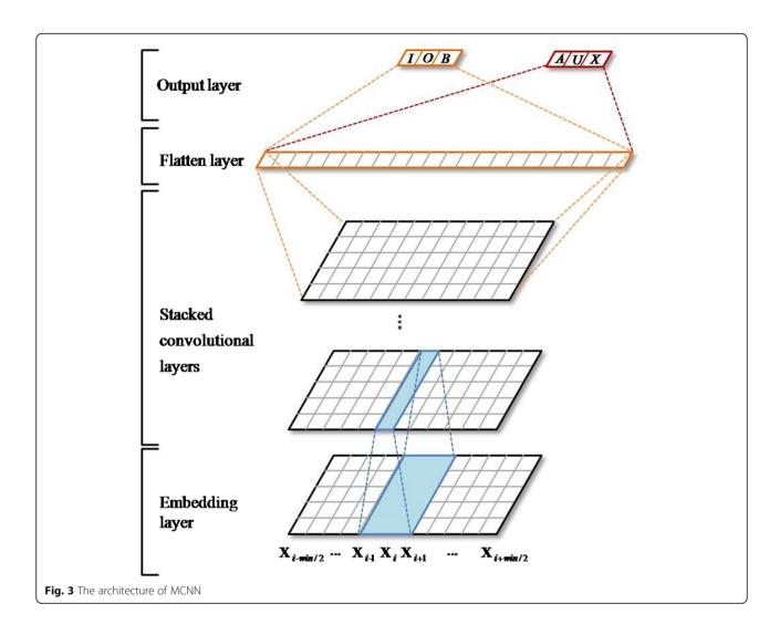
full-connected output layer is stacked over the flatten layer and obtains the output vectors:  $\begin{aligned} & out^{main} \\ & = \left[out_1^m, out_2^m, ..., out_z^m\right] \end{aligned} \quad \text{and} \quad \begin{aligned} & out^{aux} \\ & = \left[out_1^a, out_2^a, ..., out_k^a\right] \end{aligned} \quad \text{where } out_i^m \text{ and } out_i^a \text{ stand for the confidence scores of the corresponding labels for the main and auxiliary outputs, respectively.}$
