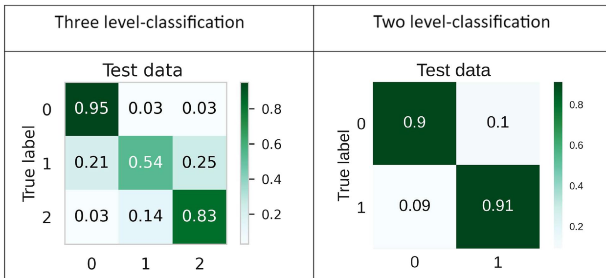
Fig. 6 Performance of developed models through Confusion-Matrix for two and three-level classification using the proposed stacking classifier
