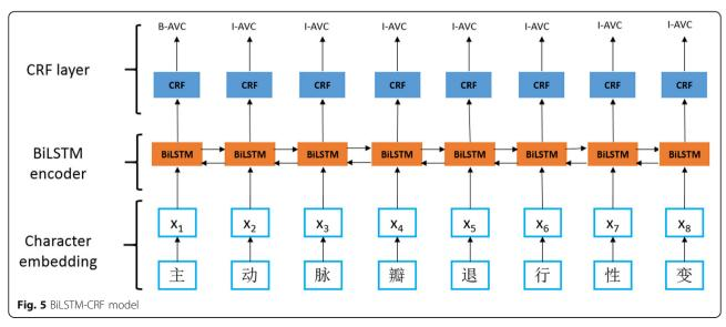
The third layer is the CRF layer, where sentence-level sequence tagging is carried out. The parameters of the CRF layer are a  $(k+2) \times (k+2)$  matrix A.  $A_{ij}$  represents the transfer score from the ith label to the jth label. If we use a sequence of labels  $y = (y_1, y_2, ..., y_n)$  which length is equal to the length of the sentence, the model scores when the label of the sentence x equals y is:
