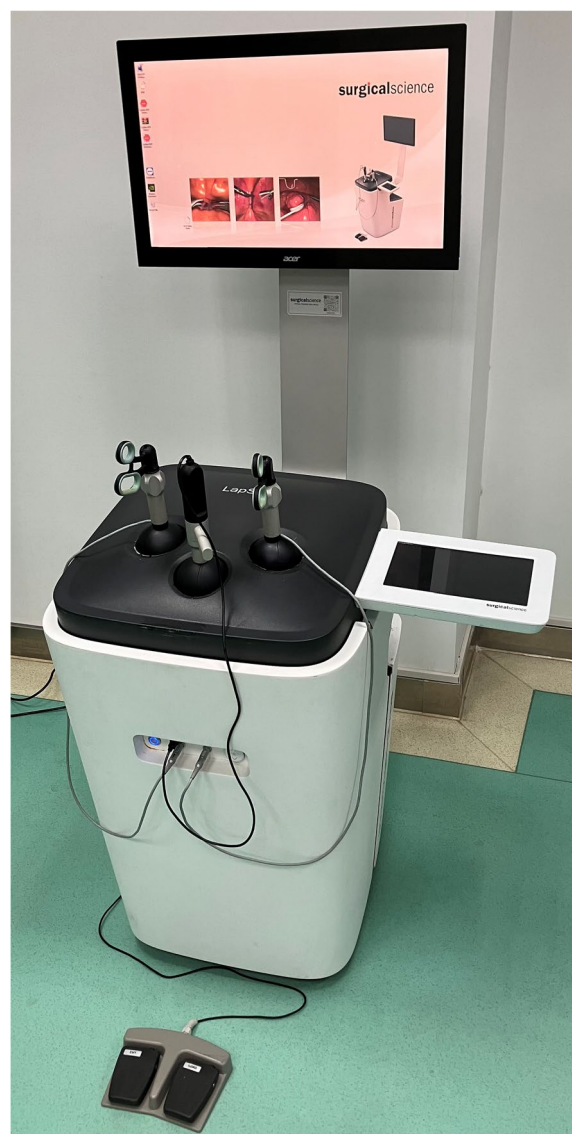
Fig. 1 The laparoscopic simulation training system
