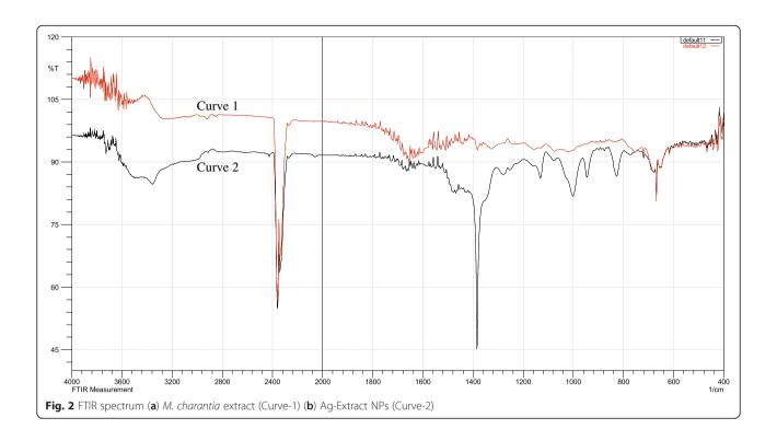
stretching. The weak band observed at 2926.01 cm<sup>-1</sup> and 2880.79 cm<sup>-1</sup> (both in curve-1 and curve-2) indicates the H-C-H asymmetric and symmetric stretching of alkanes. The band observed at 2341.58 cm<sup>-1</sup> (curve-1) and 2368.94 cm<sup>-1</sup> (curve-2), which are very nearer band, denotes the presence of hydrogen bonded OH stretching of carboxylic acids in leaf extract which may be a reducing/coating agent for silver nanoparticles.
