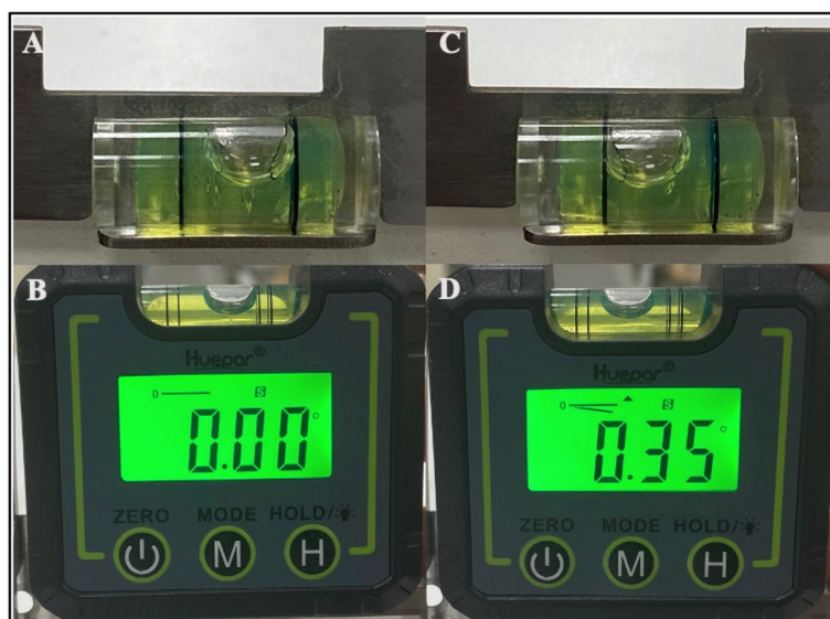
Fig. 1 Verification assessment of the OCIT by detecting the accuracy of the bubble level, A the bubble in touch with the right mark, B reading of the digital angle gauge, C the bubble in touch with the left mark, D reading of the digital angle gauge
