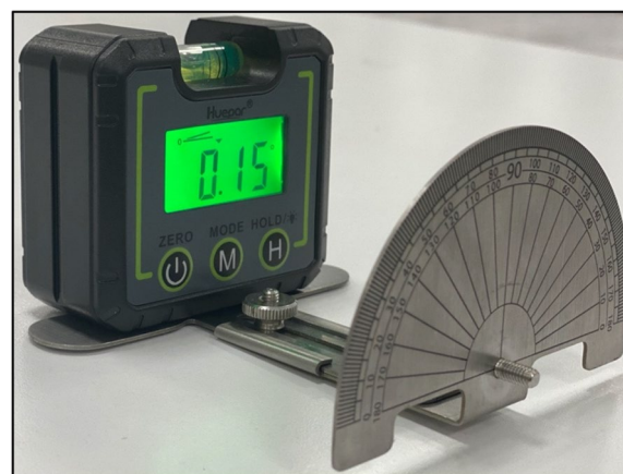
Fig. 2 Verification assessment of the OCIT by evaluating the relationship between the bite plate and the protractor
