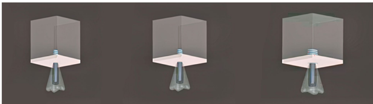
Fig. 2 Buttress thread models of 4 mm (left), 5 mm (middle), and 6 mm diameter (right)
