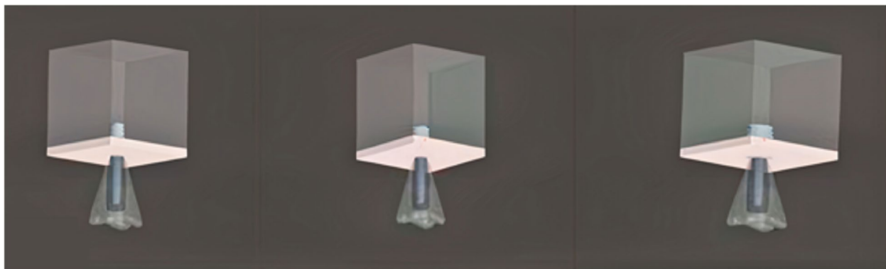
Fig. 4 Triangular thread models of 4 mm (left), 5 mm (middle), and 6 mm diameter (right)
