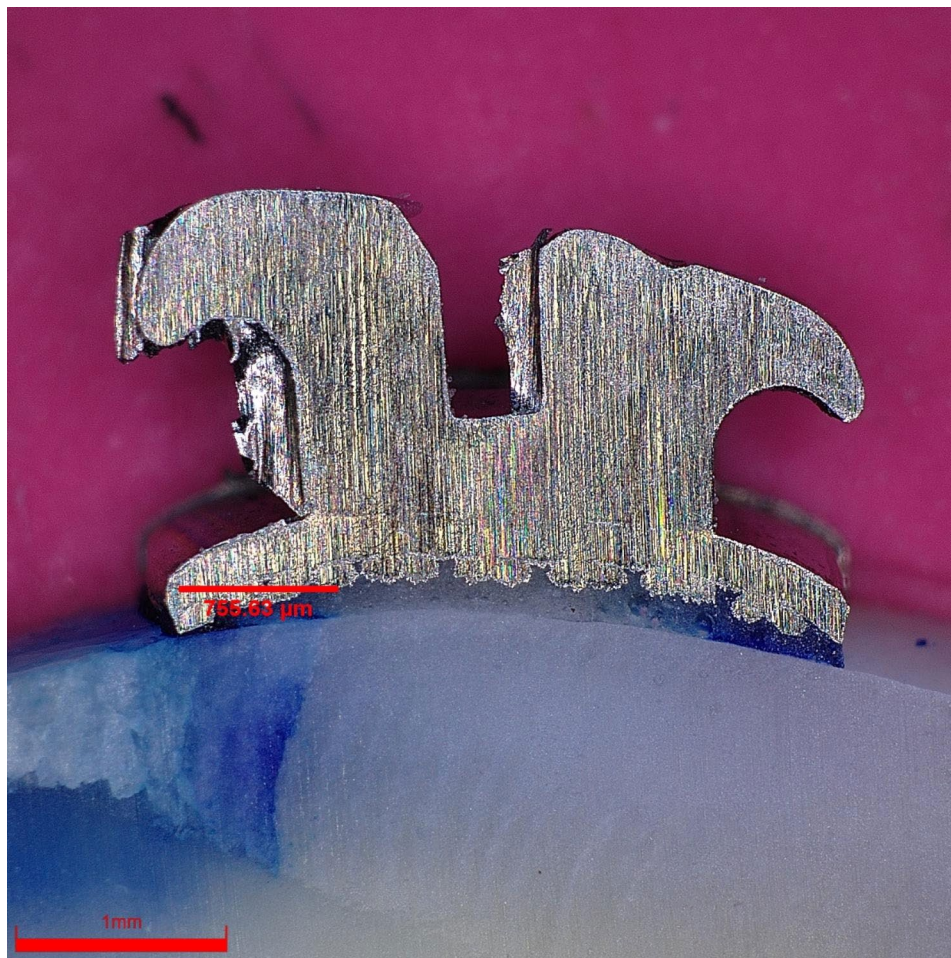
Fig. 1 A magnified view (60 \times ) of a section of a metal orthodontic bracket (Legend medium metal bracket by GC Orthodontics) with methylene blue staining indicating microleakage between the adhesive material Transbond XT (by 3 M Unitek) and enamel. The image was captured using a digital microscope (OLYMPUS DSX 1000)
