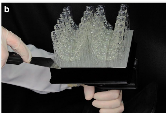
Fig. 3 a Ten identical surgical guides were printed using a clear photoreactive resin material b 3D-printed surgical guides were removed from the build platform using a removing tool
