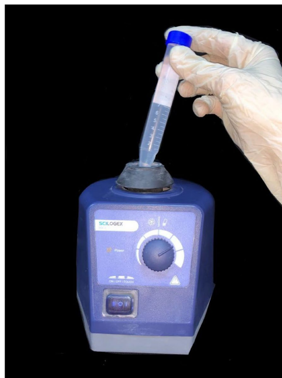
Fig. 4 15 ml Falcon tube filled with sterile distilled water and placed on the Scilogex Vortex Mixer
