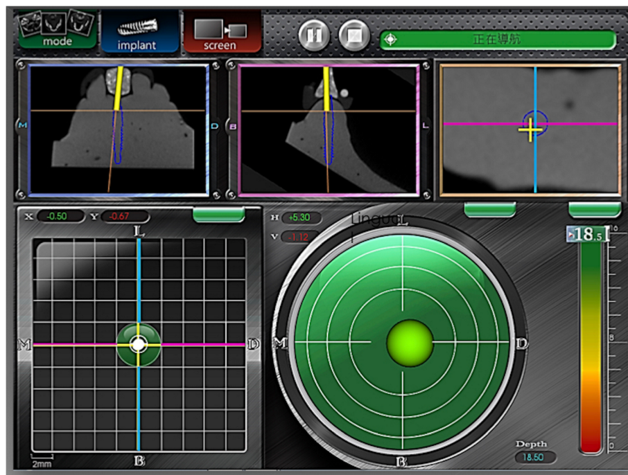
Fig. 5 Navigation monitor showing real-time implant drilling. Three-dimensional (3D) image monitor helps surgeon to correct the error immediately
