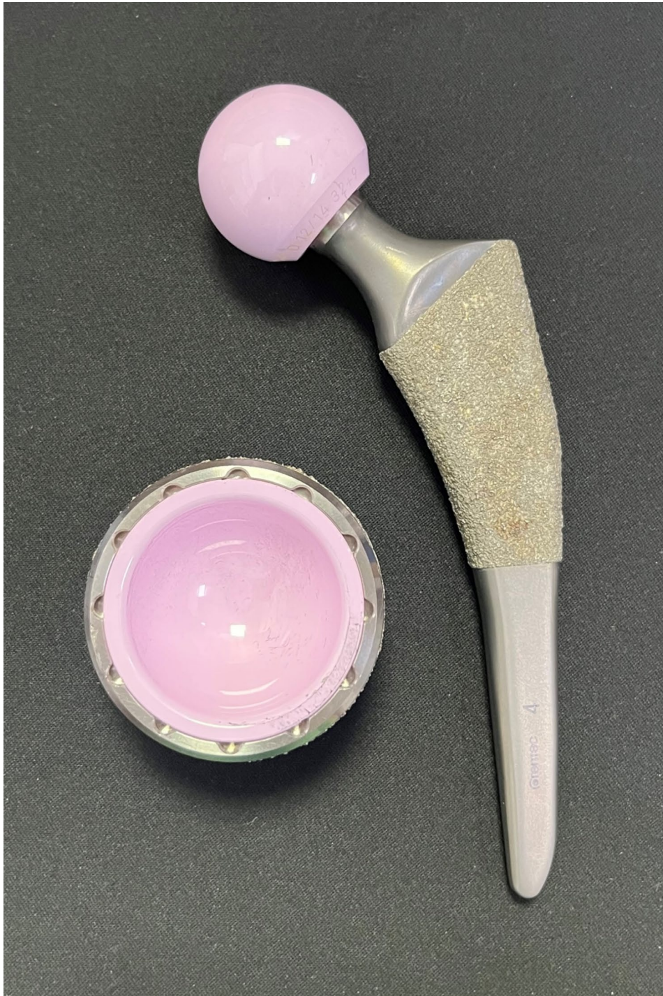
Fig. 2 Bencox Mirabo cup with M femoral stem (Corentec, Cheonan, Korea) and BioloX Delta bearing (Ceramtec, Plochingen, Germany) were used in this study
