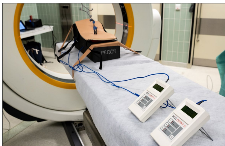
Fig. 3 Experimental setup of model in prone position and Conny II devices
