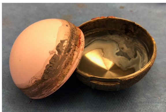
Fig. 9 The acetabular shell and the ceramic liner taken apart and showing important signs of wear and corrosion debris on the taper surfaces
