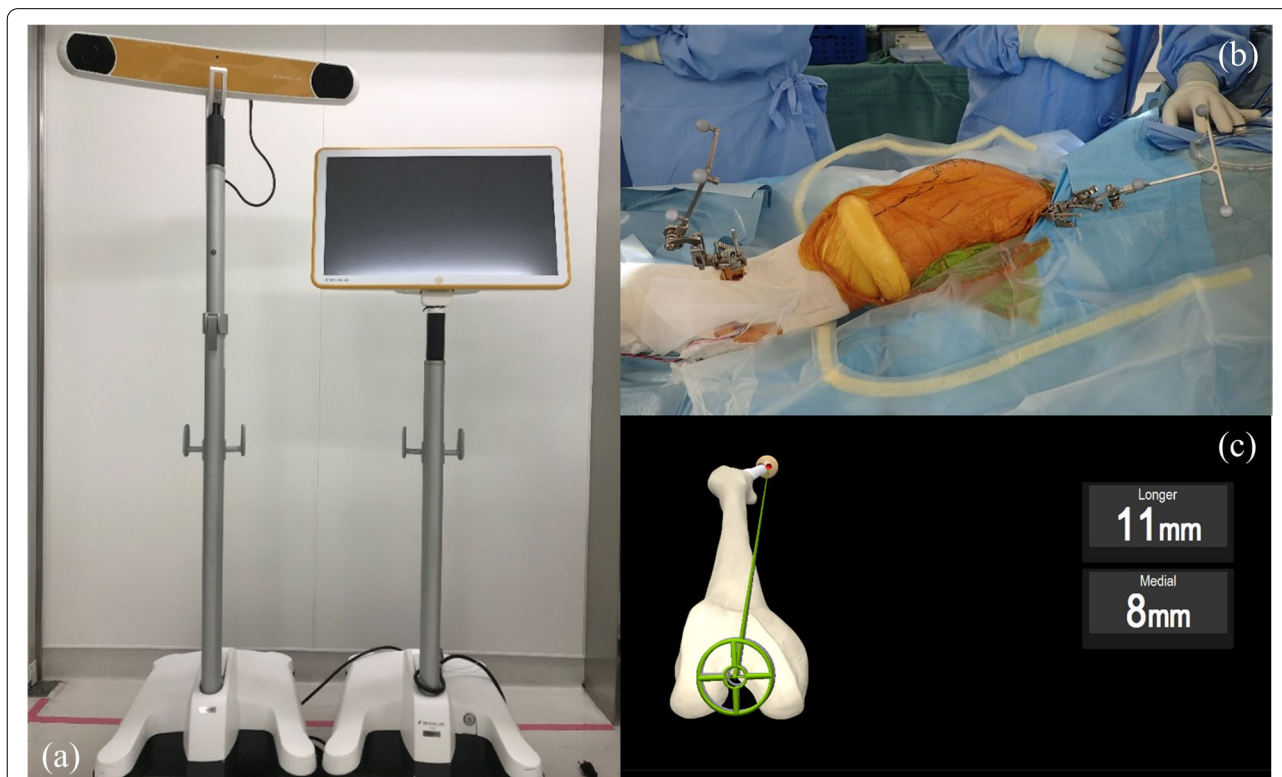
Fig. 1 a The image-free navigation system (Brain Lab, KICK Hip application 6.0, Helmstetten, Germany). b Setting position of trackers on the pelvis and distal femur with two pins each. c Monitor image showing intraoperative leg length and offset values
