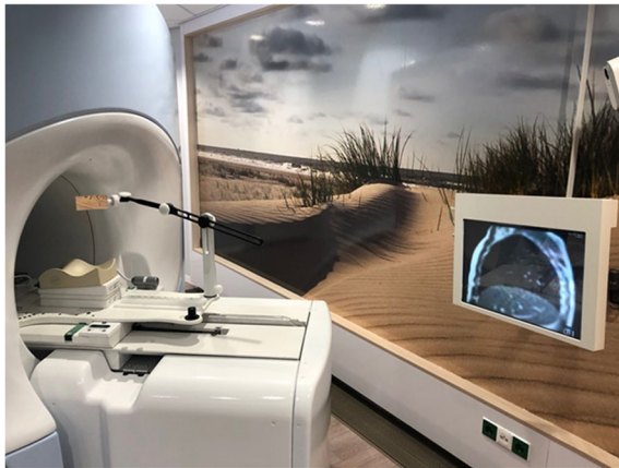
Fig. 2 The visual feedback system, including an MR-compatible monitor at the head end of the MR bore and an adjustable mirror (Botman et al., Clin Transl Radiat Oncol. 2019)
