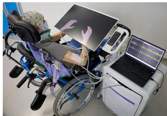
Fig. 2 DiSCloser BCI station. The Brain-Computer Interface training station developed for patients with Spinal Cord Injury to practice the kinaesthetic motor imagery of hand closing and opening in a close-loop condition. The system is equipped with a laptop, a commercial wireless EEG/EMG system and a screen for the ecological feedback to the participant. The ecological feedback is delivered by means of a custom software program that provides for (personalized) visual representation of the participant's own hands. The screen for the feedback is adjustable in height and tilt to adapt to use in wheelchair or bed. The participant in the photo filled out the photo release consent form
