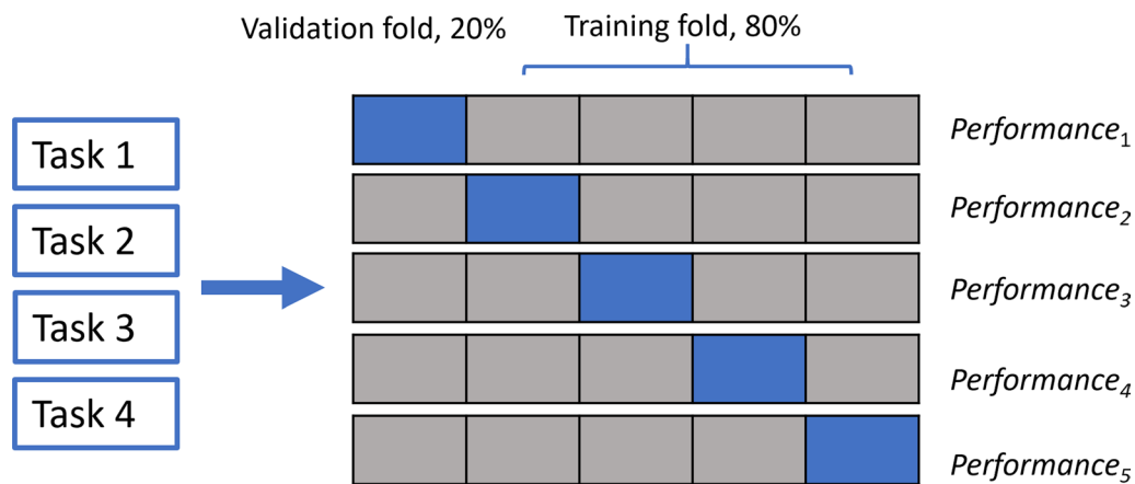
Fig.5 Training and validation workflow of each DL model for grade classification
