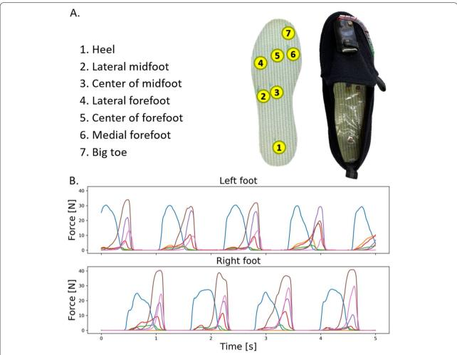
**Fig. 1** Overview of the 7-sensor plantar pressure measurement insole device and output. **A**: Seven pressure sensors are inserted in a 2 mm-thick hygienic shoe insole. The insole is inserted in a commercial Velcro shoe, and the data acquisition unit is attached using an additional piece of Velcro on the tong. **B**: A five-second example of plantar pressure data was collected from a walking test
