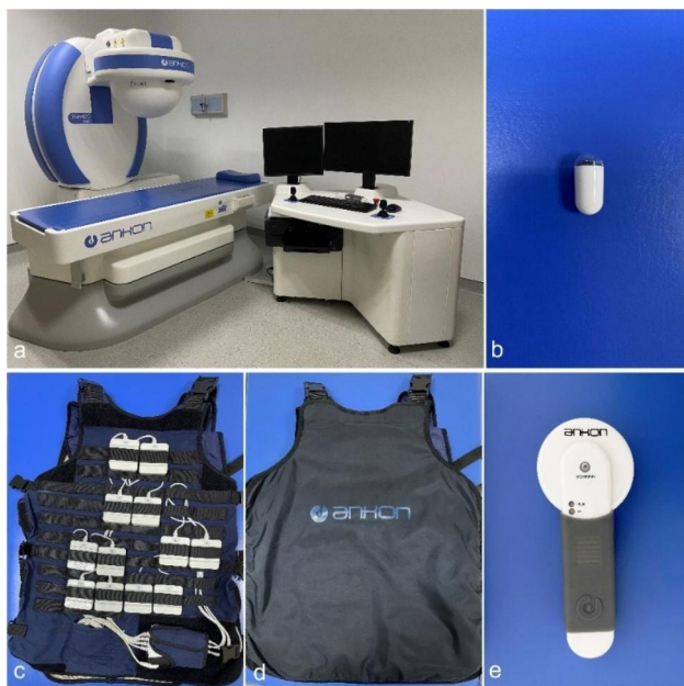
Fig. 2 The MCE system, (a) Guidance magnetic robot and a computer workstation with ESNavi software, (b) Endoscopic capsule (11.8 × 27 mm), c&d. Data recorder (check suit), e. Detector
