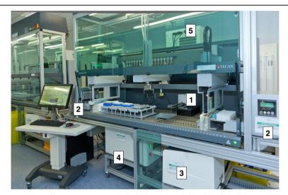
**Fig. 1** UK Biobank DNA Extraction System. This system comprises 1) Ziath® DataPaq High Speed Single Rack Scanner ZTS-A6 for sample tracking, 2) two modified hemi-skinned Promega Maxwell® 16 instruments for DNA extraction, 3) Trinean DropSense™ 96 for DNA quantification, 4) Brooks Tube Auditor™ for volume measurement and 5) Liconic STX44 Automated Incubator to keep DNA at 4 °C after extraction
