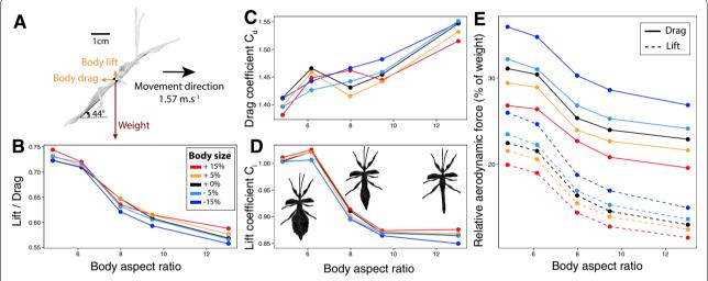
**Fig. 6** The effects of body shape on body aerodynamics as predicted by computational fluid dynamics simulations. **A** Diagram of the forces applying upon the modelled flying male leaf insect. Lift to drag ratio (**B**), drag (**C**) and lift (**D**) coefficients, drag (**E**, solid) and lift (**E**, dashed) forces relative to body weight as a function of model aspect ratio as estimated from the CFD simulations. Colors correspond to different body sizes relative to the original model
