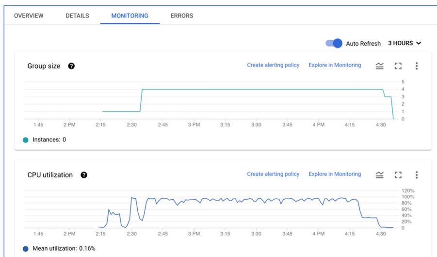
Fig. 7 Cluster size (top) and CPU utilization of the cluster (bottom) for an ElasticBLAST run with four instances. This is a screenshot of the GCP monitoring view for the cluster. The cluster has only one instance from 2:15 to 2:40 (top graph), allowing for the installation of software and databases. The bottom graph shows that the cluster has about 50% CPU utilization after 4:20, and the top graph shows the cluster size shrinking about 10 min later. The CPU utilization at a given time is based on the size of the cluster at that point in time
