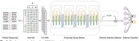
Fig. 1 The framework of the pSuc-EDBAM model
