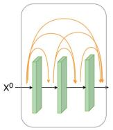
Fig. 2 The structure of a dense block
