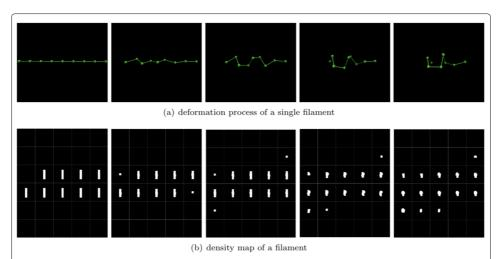
**Fig. 13** The deformation of a filament. In this figure, a single filament deforms under force field. Subfigure (**a**) shows the 3D ball-stick view, and subfigure (**b**) shows the corresponding 2D density map slice with 36 pieces. During deformation, the angle between two bonds is flexible, so that the filament can curl effectively and change its shape. Limited by the chemical bonds' length, the filament cannot be stretched
