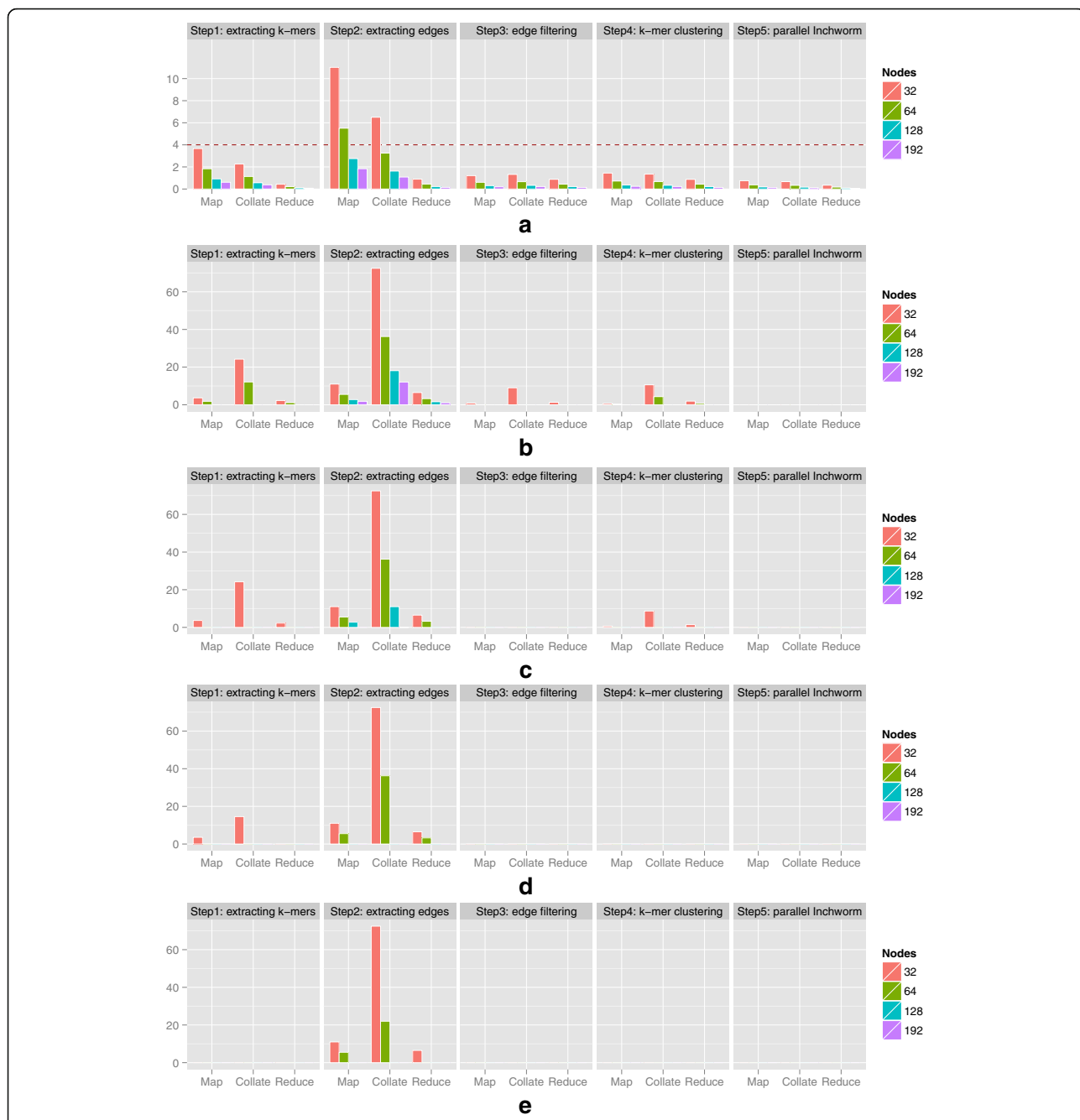
Fig. 6 Data objects created by MapReduce-Inchworm for the experimental mouse dataset (see Table 1). (a) The size of data objects generated by each MapReduce function on each compute node, as calculated from the number of KV/KMV pairs involved. The data sizes for each MapReduce function ( map() , collate() , and reduce() ) were averaged over nodes and iterations within each of the 5 main steps of MapReduce-Inchworm. (b-e) The corresponding cumulative I/O to disk, due to out-of-core processing, per compute node. Results are shown with pagesize set to: (b) 1 GB, (c) 2 GB, (d) 3 GB and (e) 4 GB. For all graphs, the Y-axis gives the data size in GB
