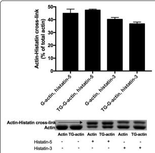
**Fig. 8** Cross-linking of 4 μM CaATP-G-actin and TGase pretreated CaATP-G-actin (TG-G-actin) with 4.5 μM Fl-histatin-3 and Fl-histatin-5 by 0.3 mg/ml TGase at 22 °C for 30 min. Preparation of TG-G-actin: 108 μM CaATP-G-actin was incubated with 4 mg/ml TGase at 4 °C for 24 h. After cross-linking samples were run on SDS-PAGE and evaluated by densitometry. *Upper panel* quantitative evaluation of SDS-PAGE by densitometry. *Lower panel* representative SDS-PAGE visualized by Coomassie blue
