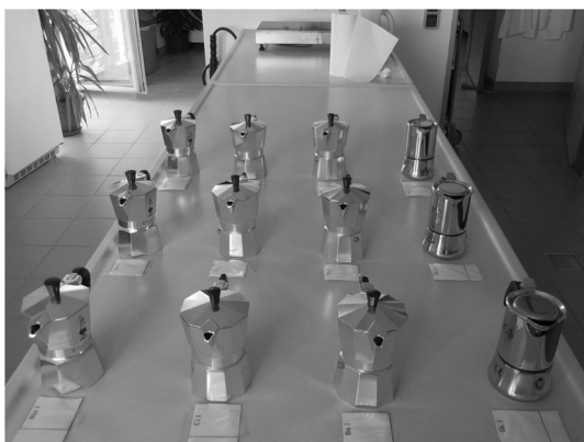
Fig. 1 The moka pots tested were made of aluminum or stainless steel (Stainless steel The right-hand row)
