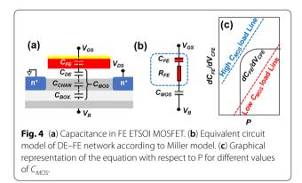
two equations with respect to time (t), an equation for  $dV_{FE}/dt$  can be derived. For ultra-steep SS characteristics,  $dV_{FE}/dt$  should change from a positive to a negative value in case of positive ramp ( $dV_{GS}/dt$  and dP/dt are positive) or negative to positive for negative ramp. Therefore, the condition for ultra-steep SS characteristics in the DE–FE network can be written as the following equation:
