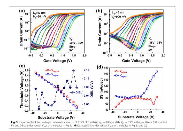
existing under high positive  $V_{SUB}$  with 50 mV  $V_D$ , the accurate minimum SS values should be higher than that shown in Fig. 3d, but it does not affect the conclusion that subthreshold characteristics improving under negative  $V_{SUB}$ .
