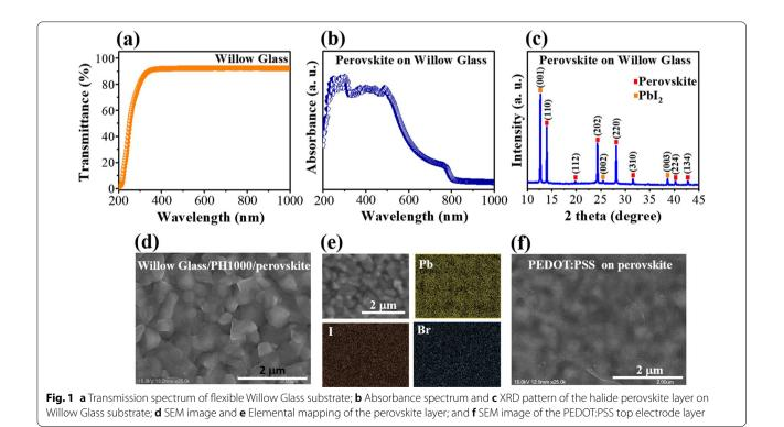
of the top electrode can be clearly observed in the SEM image in Fig. 1f. It confirms a 100% surface coverage on the prior layer by the prepared PEDOT:PSS solution via a simple spin-coating method.
