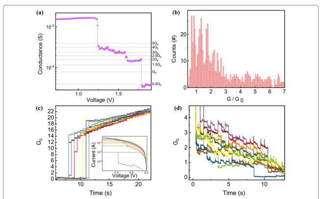
**Fig. 5** a Quantized conductance characteristic using DC measurement on reset part, and **b** histogram of quantized conductance levels. Quantized conductance characteristic using pulse measurement **c** in set region, **d** in reset region
