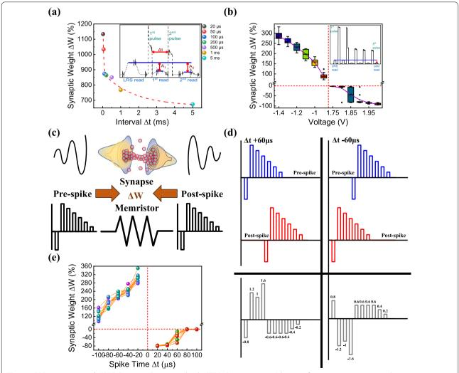
Fig. 7 a PPD measurement, **b** EPSC data according to amplitude. STDP characteristics: **c** Schematic for measurement imitation between synaptic neural structure and RRAM, **d** pulse authorization for STDP measurement at  $\Delta t = 60 \, \mu s$  and **e** result of STDP measurement
