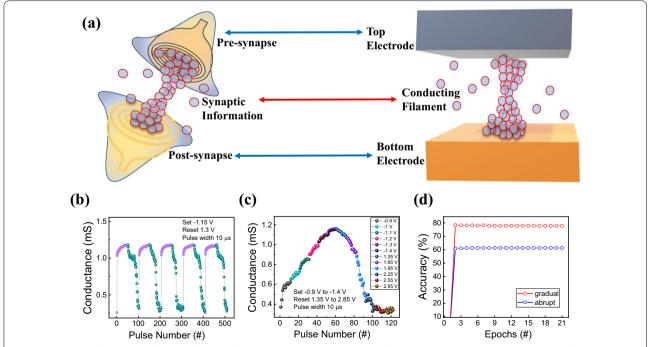
**Fig. 6** a Schematic illustration of similarity between human synaptic neural structure and RRAM device structure. Potentiation and depression characteristics: **b** consecutive same voltage pulse, **c** single incremental voltage pulse. **d** MNIST pattern recognition simulation results of (**b**) and (**c**)
