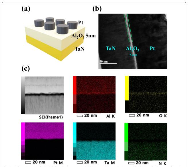
**Fig. 1** a Schematics image of Pt/Al $_2$ O $_3$ /TaN device, **b** cross-sectional TEM image, **c** EDS mapping images of Pt, Al, O, Ta and N elements collected from the area indicated in the TEM image of the Pt/Al $_2$ O $_3$ /TaN device
