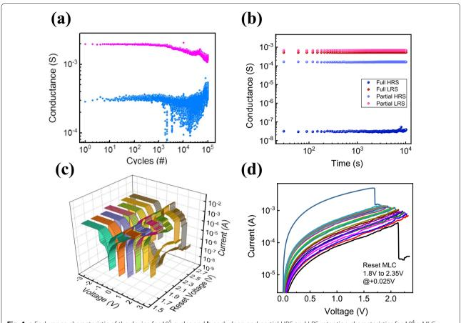
**Fig. 4** a Endurance characteristic of the device for  $10^5$  cycles and **b** each deep and partial HRS and LRS retention characteristics for  $10^4$  s. MLC characteristics of **c** different reset voltages, **d** consecutive incremental voltage repetition
