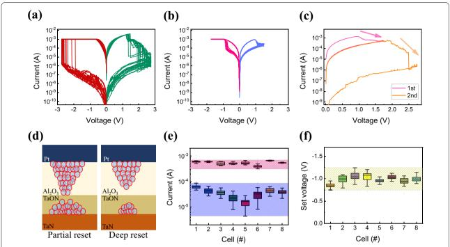
**Fig. 3** Bipolar resistive switching of Pt/Al<sub>2</sub>O<sub>3</sub>/TaN device: **a** deep reset, **b** partial reset, **c** process of inducing from partial reset to deep reset, and **d** deep and partial reset mechanism schematic diagram. Uniformity of **e** HRS and LRS, **f** set voltage
