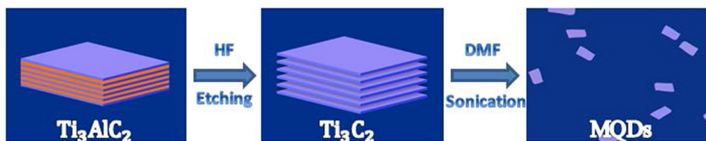
Fig. 1 Schematic diagram for the preparation of MQDs
