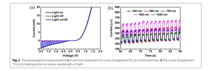
(350–1050 nm). The photoresponse currents ( $I_{on} - I_{off}$ ) at 350, 55, 750, 950, and 1050 nm are 126.29, 213.35, 189.67, 335.93, and 102.46  $\mu$ A, respectively.
