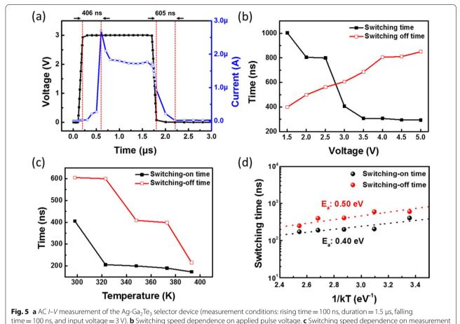
temperature. **d** Arrhenius plot of switching speed against measurement temperature
