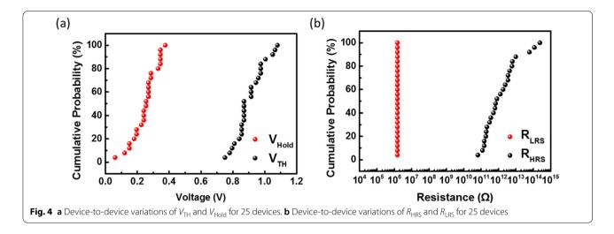
resistance distribution at the HRS ranged from  $10^{11}$  to  $10^{14} \Omega$ , while the resistance at the LRS was approximately  $10^{6} \Omega$ , as shown in Fig. 4b. Owing to the metal conduction channel formation, selector devices using active metals such as Ag or Cu exhibit relatively wide variation characteristics [36, 37]. Accordingly, studies on improving the reliability of these characteristics via doping or buffer layer insertion have been reported [37, 38].
