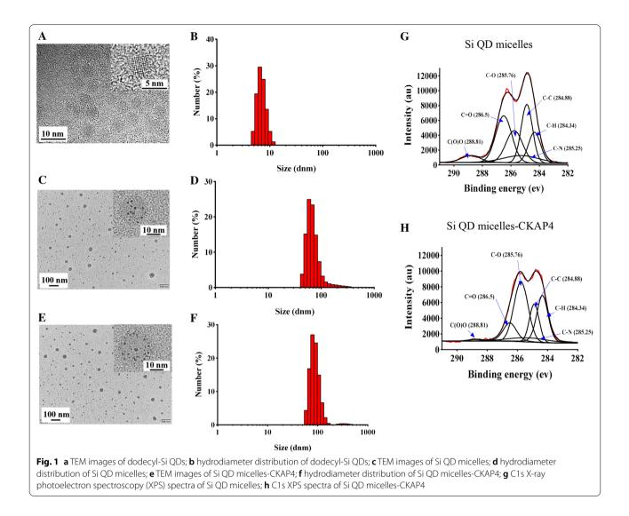
Data showed that the average distance between lattice fringes is approximately 0.35 nm, which is nearly the same as that of the previously reported dodecyl-Si QDs (0.34 nm). Therefore, the dodecyl-Si QDs synthesized in this study showed good crystallinity [12]. Dynamic light scattering (DLS) showed the hydrodynamic diameters of dodecyl-Si QDs ranging from 4.8 to 13.5 nm with an average of 6.5 nm (Fig. 1b).
