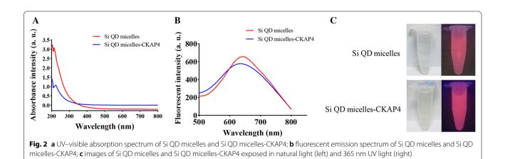
conjugation exerted no significant influence on the fluorescence properties of the Si QD micelles-CKAP4. The Si QD micelles-CKAP4 aqueous solution (Si concentration:  $80 \mu g/mL$ ) was transparent and clear in natural light. Under 365 nm UV light, it could emit strong red fluorescence, consistent with the results of the Si QD micelles (Fig. 2c). PL QY tests showed that the absolute PL QY of the Si QD micelles-CKAP4 was approximately 16.96%.
