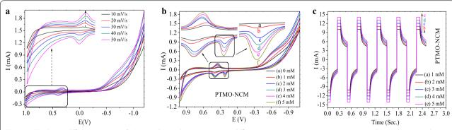
Fig. 5 a CV plots at different scan rates. b CV ascorbic acid sensing curve at different concentrations. c Amperometric ascorbic acid sensing plot at different concentrations
