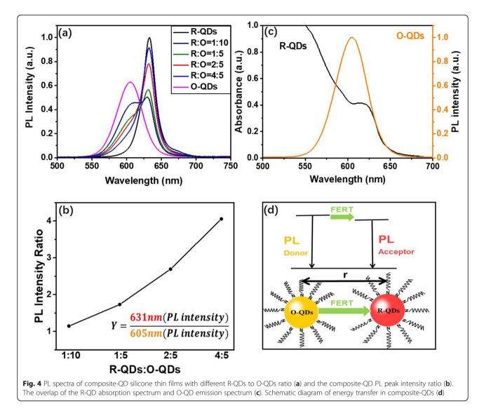
in Fig. 4b. The peak intensity ratio presents a rising increment with the R-QD percentage, which suggests the energy transfer from O-QDs to R-QDs. Figure 4c exhibits the overlap between the R-QD absorption spectrum and the O-QD emission spectrum. It suggests a high chance of FRET process, in which the O-QDs acts as the donor and R-QDs as the acceptor (shown in Fig. 4d).
