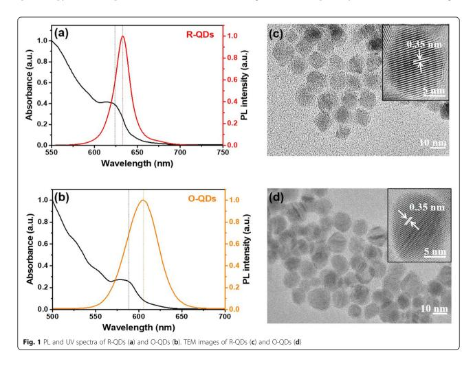
show an interplanar distance of 0.35 nm, which can be assigned to the (111) plane of the cubic phase ZnS.
