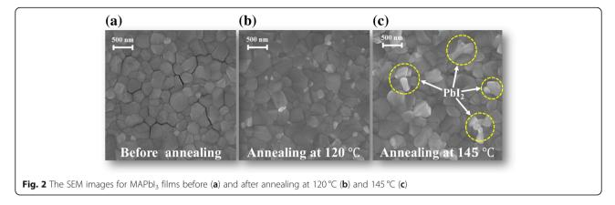
From these findings, we can conclude that a compositional change could occur in the MAPbI<sub>3</sub> film annealed above 145 °C. By releasing the organic species during annealing, PbI<sub>2</sub> components are decomposed and parts of them are located at the perovskite GBs according to both XRD and SEM results.
