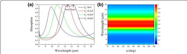
**Fig. 2** Absorption spectra at the normal incidence with different  $E_F$  at  $\varphi = 0$ , showing large blueshift of the peaks with increasing  $E_F$  (**a**), and with different  $\varphi$  at  $E_F = 0.2$ eV, demonstrating a polarization independence (**b**). The polarization angle  $\varphi$  is defined as in Fig. 1a
