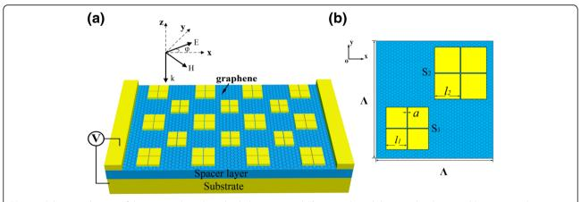
Fig. 1 a Schematic diagram of the proposed graphene-loaded metamaterial. The cross-shaped slot in each subunit enables a great enhancement of graphene-light interaction without polarization dependence. b Top view of the structure in one period. Two subunits are arranged diagonally with different patch sizes
