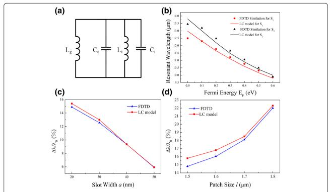
**Fig. 4 a** An LC circuit model includes contributions from separate patches ( $L_a$ nd  $C_i$ ), slot ( $C_c$ ), and graphene ( $L_g$ ). **b** Resonances calculated by the LC model compared with FDTD simulations. **c**, **d** Resonance shift for a single patch at  $E_F = 0.4$  eV with changing geometrical parameter of **c** slot width ( $I = 1.5 \mu m$ ) and **d** patch size ( $I = 2.0 \mu m$ )
