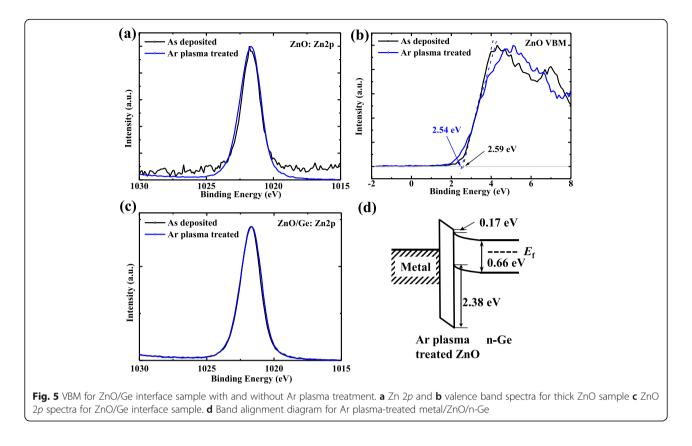
more pronounced in comparison with the as-deposited sample, indicating that more  $V_{\rm o}$  are generated due to Ar plasma treatment, and chemisorbed oxygen is effectively removed. The increasing of n-type dopants in ZnO results in the thinner tunneling barrier and lower series resistance at interface, being responsible for the reduction in  $R_{\rm c}$  [36].
