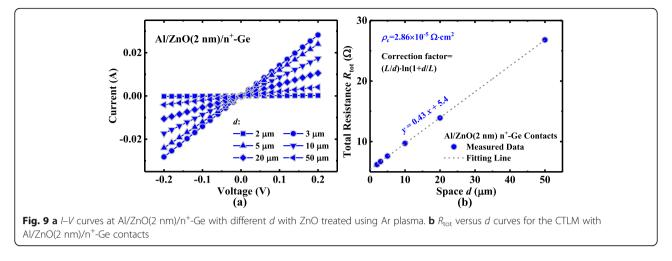
treatment achieves the enhanced *J* compared to the device with 2 nm ZnO or 3 nm ZnO, which is due to that a large amount of  $V_{\rm o}$  are generated in ZnO film during the Ar plasma treatment. The higher doping concentration in ZnO can effectively reduce the series resistance of ZnO and reduce the tunneling barrier for electrons at the interface between ZnO and Al, improving the tunneling current density.
