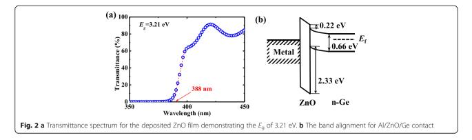
and Ge 3*d* peak position for ZnO/Ge interface sample are 1021.7 eV and 29.1 eV, respectively. The Ge 3*d* peak position and VBM for pure Ge sample are 29 eV and 0.06 eV, respectively. This indicates that the VBO of ZnO/Ge is 2.33 eV [30].
