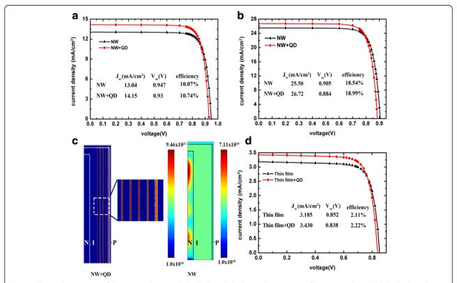
Fig. 5 a The I-V characteristics of short NW and NW/QD hybrid solar cells. b The I-V characteristics of long NW and NW/QD hybrid solar cells. c Half of the vertical cross section of radiative recombination rates of short NW and NW/QD hybrid solar cells. d The I-V characteristics of thin-film and thin-film/QD hybrid solar cells
