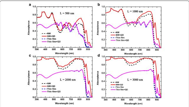
Fig. 3 The absorption spectra of the NW/QD hybrid nanostructure array and its thin-film counterpart with and without QD layers. The NW length in a-d is 500, 1000, 2000, and 3000 nm, respectively
