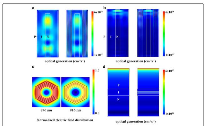
Fig. 4 a The vertical cross section of optical generation profiles in short NW and NW/QD hybrid solar cells. **b** The vertical cross section of optical generation profiles in long NW and NW/QD hybrid solar cells. **c** The electric field distributions in NW cross section at 876 and 916 nm, in which the location of QD layers is marked out with white lines. **d** The vertical cross section of optical generation profiles in thin-film and thin-film/QD hybrid solar cells
