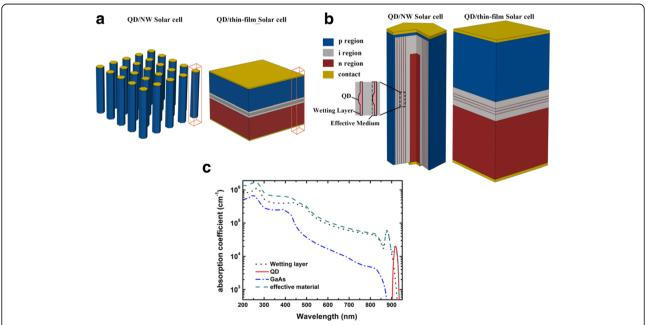
Fig. 1 a The schematic drawings of the NW/QD hybrid solar cell and its thin-film counterpart. b The detailed structures of the units marked with wireframes in a. c Absorption coefficient of the effective medium. The volume fractions of QDs, WL, and GaAs in the effective medium are 0.002882996, 0.649123, and 0.347994, respectively
