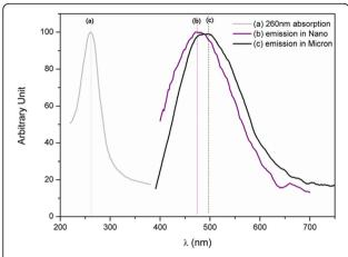
**Fig. 2** Photoluminescence of Ti-doped MgAl $_2$ O $_4$ : **a** 260 nm excitation, **b** nano, and **c** micron [12] powders synthesized at 500 °C, 1 h, and 1300 °C, 2 h, respectively
