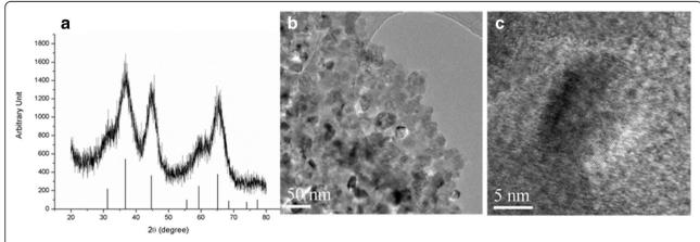
Fig. 1 a XRD pattern for Ti-doped nano MgAl<sub>2</sub>O<sub>4</sub> powder synthesized at 500 °C 1 h with reference peaks of MgAl<sub>2</sub>O<sub>4</sub> from JCPDS and **b**, **c** TEM images of the powder
