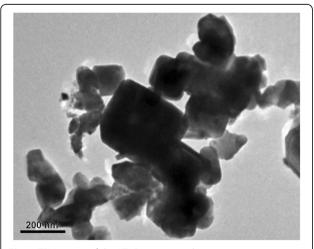
Fig. 4 TEM image of the KTaO<sub>3</sub> nanoparticles
