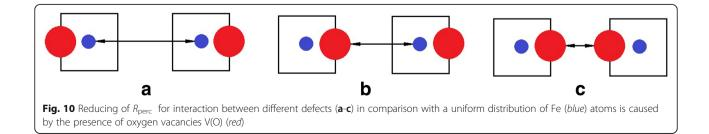
cases,  $R_{perc}$  can be defined as the distance V(O)-Fe or V(O)-V(O) from different cells (see Fig 10b, c). When the number of V(O) increases, the number of cases presented in Fig. 10b, c also increases, respectively. Accordingly, the calculated value of b = 0.25 nm indicates that mainly an exchange interaction occurs directly between the electrons trapped in oxygen vacancies.
