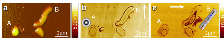
Fig. 9 AFM and MFM measurements. AFM (a) and MFM (b, c) images of vertically (A) and horizontally (B) aligned fragments of ZnO:Mn (15%) nanorode. Arrows indicate direction of MFM tip scanning. Inserts in b and c show model sketches of magnetic domains
