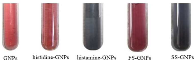
Fig. 5 Interaction between GNPs with fresh chicken meat sample (FS) and spoiled sample (SS)
