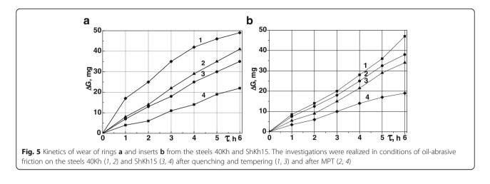
The wear resistance of steels 40Kh and ShKh15 after MPT is higher than the same steels after quenching and low tempering which are confirmed by wear resistance investigations (Fig. 5a). It should be noted that formed during MPT oxides FeO and Fe<sub>3</sub>O<sub>4</sub>, being secondary structures could also decrease wear by the way of relieve running-in of the friction pairs [16].
