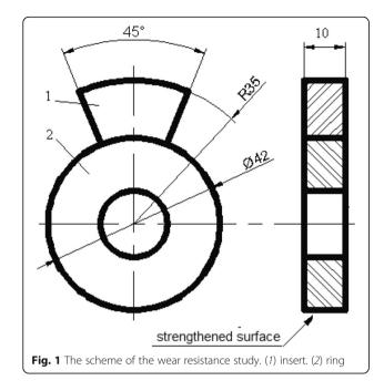
The same scheme was used to establish the friction coefficient in air and in oil without addition of quartz sand. The insert-specific pressure on the ring varied between 2.0 and 6.0 MPa.
