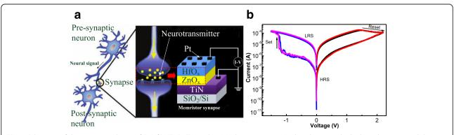
**Fig. 1** Schematic of the memristor device of Pt/HfO<sub>x</sub>/ZnO<sub>x</sub>/TiN and its *I–V* characteristics. **a** Analogy between the biological synapse and the electronic synapse based on the Pt/HfO<sub>x</sub>/ZnO<sub>x</sub>/TiN memristor device. **b** *I–V* characteristics of the Pt/HfO<sub>x</sub>/ZnO<sub>x</sub>/TiN synapse device measured by a typical DC double sweep
