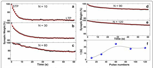
**Fig. 5** The memory retention for synaptic weight of  $Pt/HfO_x/ZnO_x/TiN$  memristive device: transformation from STP to LTP induced by repetitive pulse stimulation. **a–e** Memory forgetting process (*black solid circle* in figure) was experienced by different numbers of pulse stimulation, in which the normalized data was fitted using Eq. 1. **f** The relaxation time ( $\tau$ ) changes with the number of pulses by fitting the data from Fig. 5(**a–e**)
