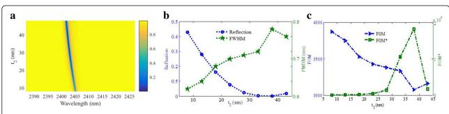
**Fig. 4 a** Reflection spectra as a function of  $t_2$ . **b** Reflectivity of the resonance dip and its FWHM as functions of  $t_2$ . **c** FOM and FOM\* as functions of  $t_2$ . Other parameters:  $p = 1200\,$  nm,  $w = 622\,$  nm,  $t_3 = 18\,$  nm, and  $t_1 = 300\,$  nm  $t_2 = 1200\,$  nm,  $t_3 = 18\,$  nm, and  $t_4 = 120\,$  nm,  $t_4 = 120\,$  nm,  $t_5 = 1200\,$  nm,  $t_7 = 120$
