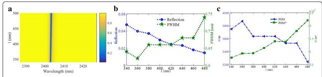
**Fig. 7 a** Reflection spectra as a function of l. **b** Reflectivity of the resonance dip and its FWHM as functions of l. **c** FOM and FOM\* as functions of l. Other parameters: p = 1200 nm, w = 622 nm, l = 420 nm,  $t_1 = 328$  nm,  $t_2 = 28$  nm, and  $t_3 = 18$  nm
