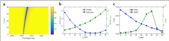
**Fig. 5 a** Reflection spectra as a function of  $t_3$ . **b** Reflectivity of the resonance dip and its FWHM as functions of  $t_3$ . **c** FOM and FOM\* as functions of  $t_3$ . Other parameters:  $p = 1200\,$  nm,  $w = 622\,$  nm,  $l = 420\,$  nm,  $t_1 = 328\,$  nm, and  $t_2 = 28\,$  nm
