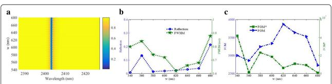
**Fig. 6 a** Reflection spectra as a function of w. **b** Reflectivity of the resonance dip and its FWHM as functions of w. **c** FOM and FOM\* as functions of w. Other parameters:  $p = 1200 \, \text{nm}$ ,  $l = 420 \, \text{nm}$ ,  $t_1 = 328 \, \text{nm}$ ,  $t_2 = 28 \, \text{nm}$ , and  $t_3 = 18 \, \text{nm}$
