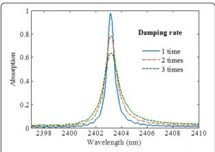
**Fig. 3** Simulated absorption spectra for damping constant of one, two, and three times that of gold
