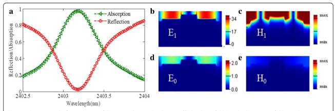
**Fig. 2 a** Absorption and reflection spectra of the proposed sensor. Distributions of **b** the electric field  $E_1$  and **c** the magnetic field  $H_1$  at the resonant wavelength. Distributions of **d** the electric field  $E_0$  and **e** the magnetic field  $H_0$  at the nonresonant wavelength. Parameters: p = 1200 nm, w = 622 nm, l = 420 nm,  $t_1 = 328$  nm,  $t_2 = 28$  nm, and  $t_3 = 18$  nm
