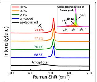
**Fig. 1** Raman spectra of samples with various P doping concentrations at the annealing temperature of 1000 °C. The *inset* is the Gauss decomposition of Raman peak
