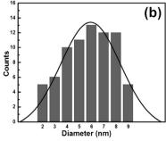
Fig. 2 a Cross-section TEM micrographs with low and high magnifications for the nominal P concentration of 0.2 % nc-Si/SiO₂ multilayers after 1000 °C annealing, b Size distribution of the nc-Si dots in the doped nc-Si/SiO₂ film
