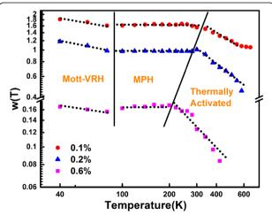
**Fig. 6** The reduced activation energy w(7) plotted against T on a log-log scale for samples with the nominal P concentration of 0.1, 0.2, and 0.6 %
