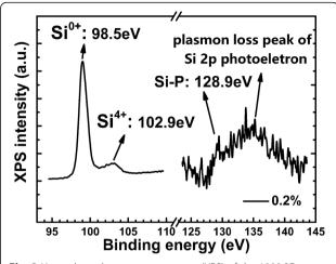
**Fig. 3** X-ray photoelectron spectroscopy (XPS) of the 1000 °C annealed samples with the nominal doping concentration of 0.2 %
