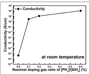
**Fig. 4** The conductivity tendency of the various P-doped nc- Si/SiO<sub>2</sub> multilavers at room temperature
