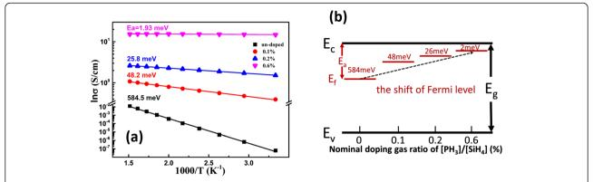
**Fig. 5 a** The Ino-1/T plot with different P doping ratios. The value listed on each line is the corresponding conductivity activation energy  $E_a$ . **b** The schematic drawing of the shift of Fermi level
