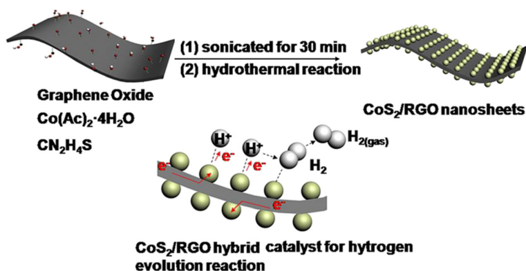
Fig. 1 Synthesis strategy and hydrogen evolution process of the CoS 2 /RGO nanocomposites
