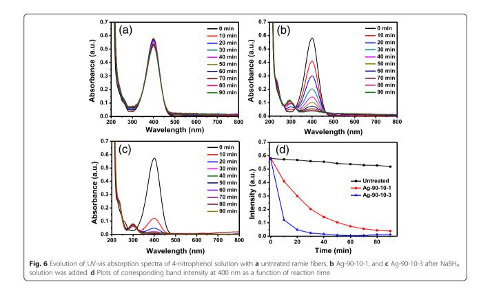
which may be due to higher silver content of Ag-90-10-3 than Ag-90-10-1. These results demonstrate that ramie fibers treated with in situ silver nanoparticles have remarkable catalytic activity for reduction of 4-nitrophenol.
